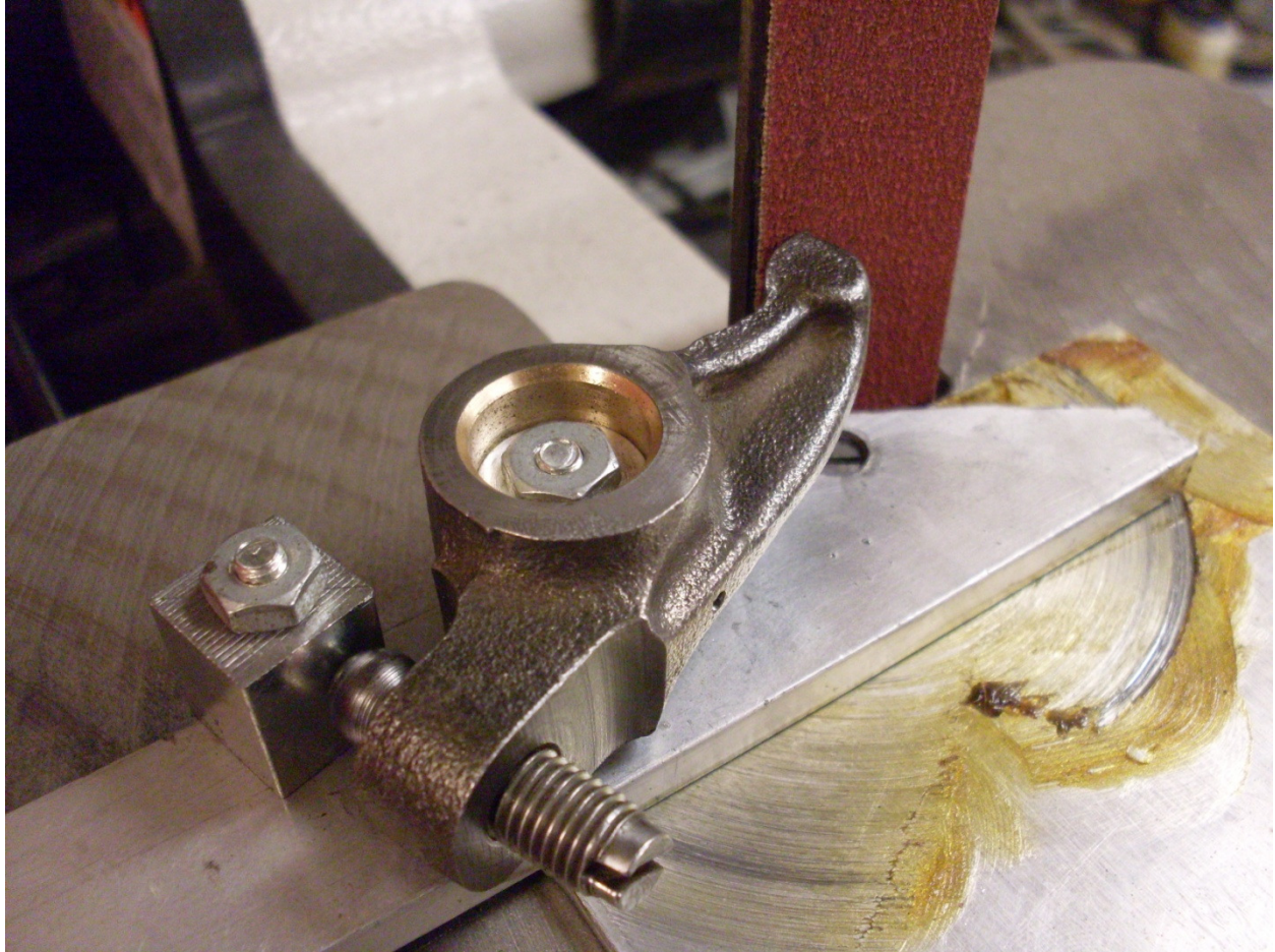
Figure 13. A rocker on the jig ready to be cut.
