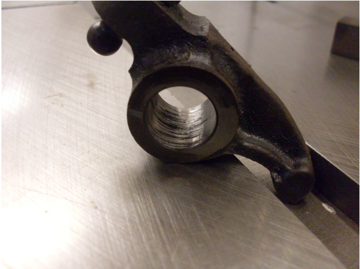
Figure 2. The rocker bores also had deep scoring.
