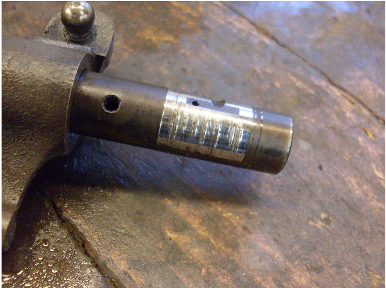
Figure 1. The rocker shaft shows pretty severe wear.
