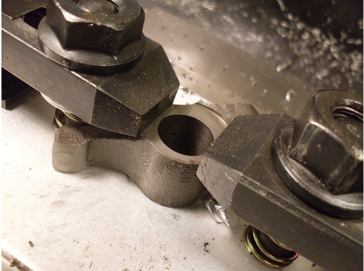
Figure 4. The rocker after being drilled and reamed to accept the bronze bush.
