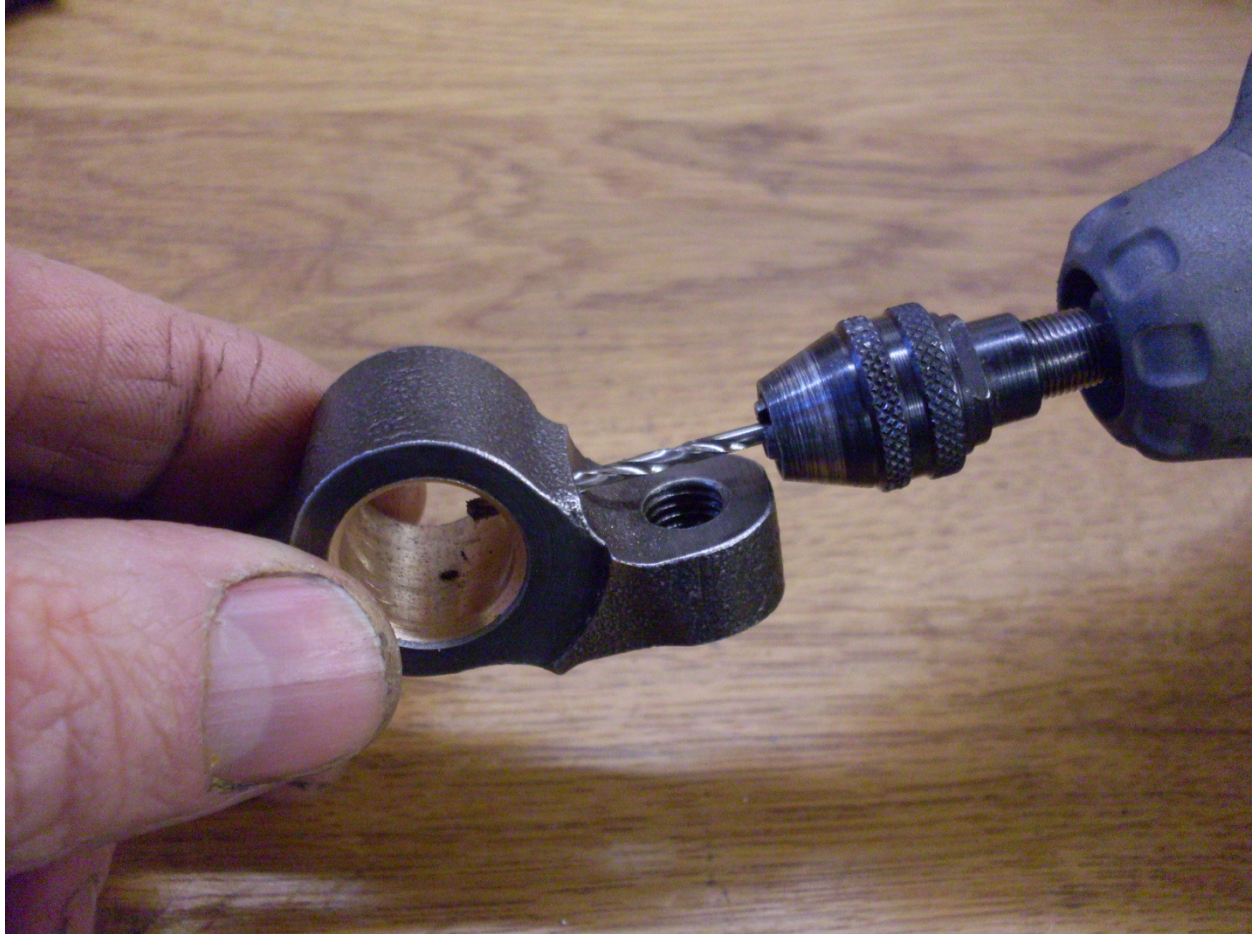
Figure 8. Drilling the oil passages through the bush.
