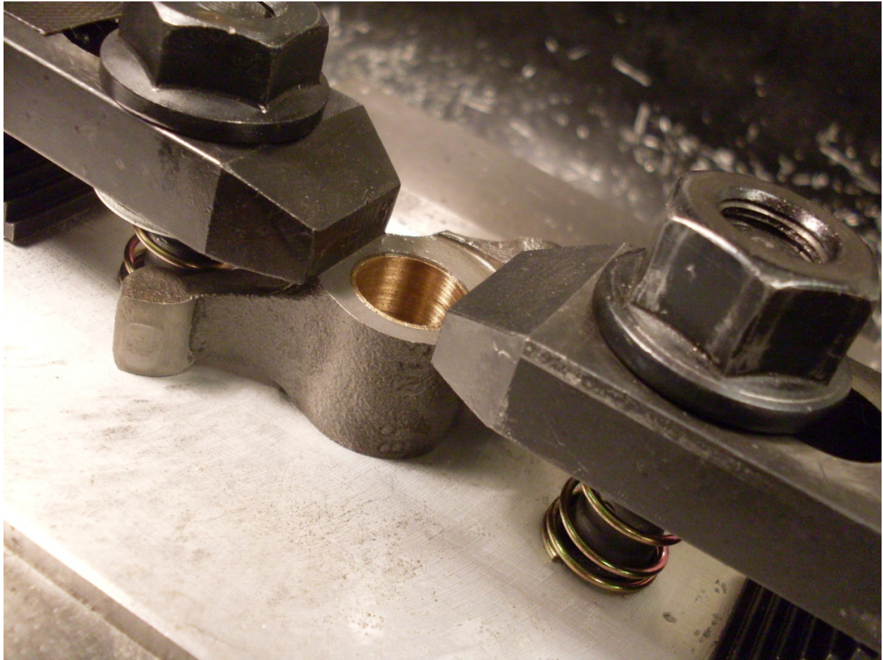
Figure 6. After the bush is drilled and reamed to fit the rocker shaft.
